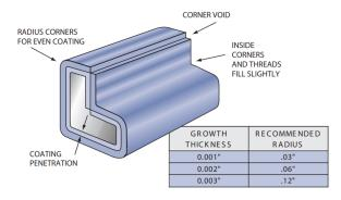
**CORNERS** - Since the coating grows (and penetrates) perpendicular to the surface of the part, sharp corners, both outside and inside, and edges can be a problem. To obtain a uniform coating, they should have a .005" to .050" radius, depending on the anodized thickness desired.
