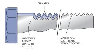
**THREADS** - The build-up on each surface changes the pitch diameter faster than typical two-surface diameters. It may be desirable to machine the threads undersize before anodizing, or mask the thread area before processing.
