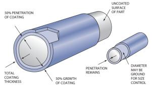
ANODIZED THICKNESS (THE 50/50 RULE) - A hard anodized finish is divided approximately 50% as a coating above the base metal (called "growth"), and 50% penetration below the surface of the part. This principle tends to hold true for most alloys and coating thicknesses.
